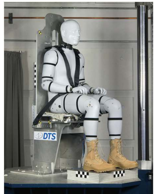
WIAMan with 146 SLICE6 HB channels
